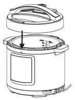
2 Align the ☐ (unlock symbol) on the lid with the ▲ on the top front of your cooker.
