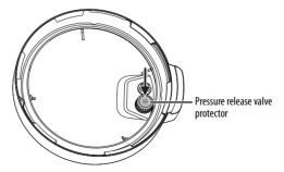
7 Install the gasket on the gasket retainer into the lid. Make sure that the gasket is correctly installed all around the retainer.
